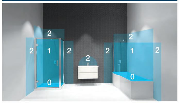
Water and electricity are a dangerous combination so when choosing bathroom lights it is essential that you familiarise yourself with two terms; Bathroom Zones and IP Ratings. When purchasing bathroom lights you need to ensure that the fitting you choose has the relevant IP rating for the Zone in which it is to be placed. So what are IP Ratings and Bathroom Zones?
